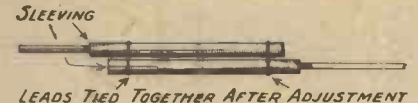
Fig. 2.—The ends of the leads which are to be tied together should be well straightened before being secured.
