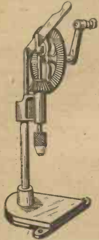
Fig. 2.—This type of bench drill, with a lever feed, is recommended to the constructor for general use.
